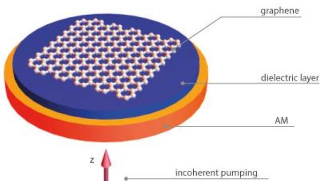
*Design of the spaser with the graphene layer shown as a honeycomb lattice above the dielectric layer (blue). The spaser is optically pumped through the active (gain) medium shown in orange.*
